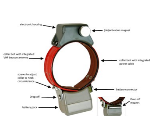
Figure 4. Vectronic GPS/GSM collar (Global Positioning System/Global System for Mobile Communications) used for telemetric monitoring of a bear
