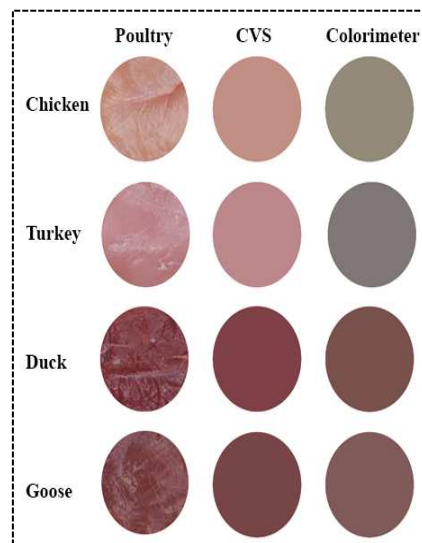
Figure 1. Color of poultry meat as measured by the two methods [1]
