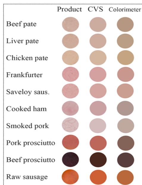
Figure 3. Color of uniformly colored meat products as measured by the two methods [2]
