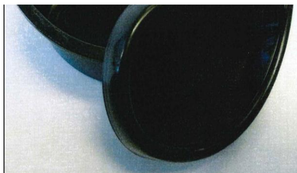
Figure 1. Examined container for pâté made from cast black colored polypropylene
