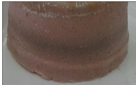
Figure 2. Discoloration of liver pâté surface that had been in contact with the polypropylene container
